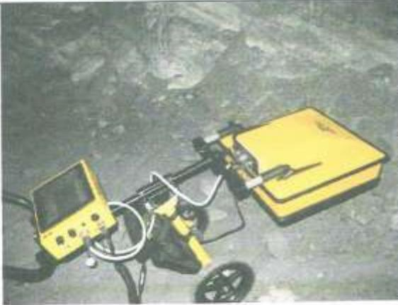
Subsurface Imaging System - Georadar
